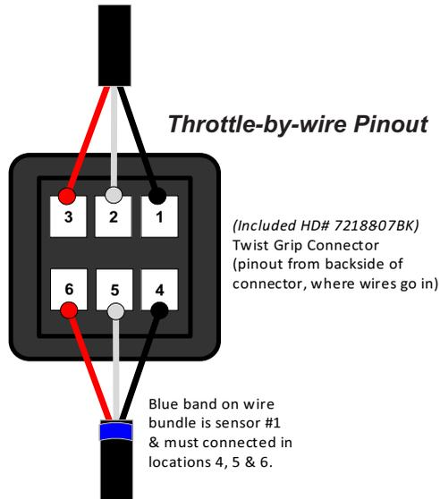
**Engine Management Harness Connector Pinout**
