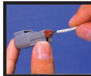
3. Push contact straight into the connector grommet until a "click" is felt. A slight tug will confirm that it is properly locked in place
